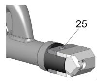
Care must be taken to ensure that the preheat nozzle provides intensive and uniform preheating (melting) of the base material over the entire joint width at as low a hot air temperature as possible. For larger weld seam widths, a wider preheat nozzle is available as an accessory.
